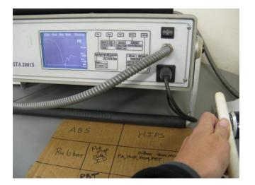
Testing plastic with laser equipment to determine type at the MBA Polymer plant in Richmond, CA. The small white pipe is held to the laser sensor and the screen reads the type, in this case it is PE.
